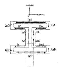
Fig.4 The equivalent magnetic current on the 2-folded slot loop antenna
