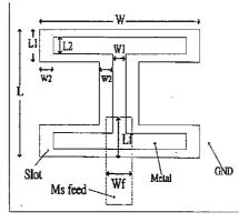
Fig.3 The antenna structure of the 2-folded slot loop antenna
