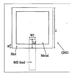
Fig.1 The antenna structure of a typical slot loop antenna
